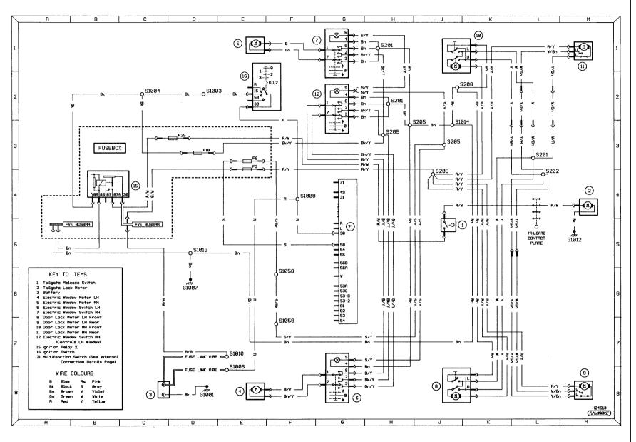
Diagram 3c: Ancillary circuits - central locking, electric windows and tailgate release (1992-on)
